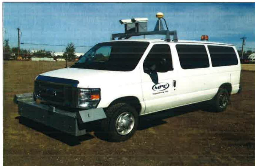
Road testing equipment used for the field data collection MPE Engineering Ltd. Pavement Testing Vehicle (Class I Profiler)
